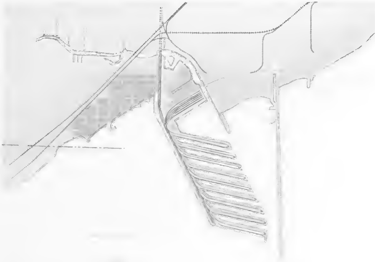
LXXII. CHICAGO. SKETCH DIAGRAM OF DOCKS SUGGESTED AT THE MOUTH OF THE CALUMET RIVER FOR BULK FREIGHT STEAMERS; ACCESS TO BE HAD WITHOUT OPENING OF BRIDGES.
